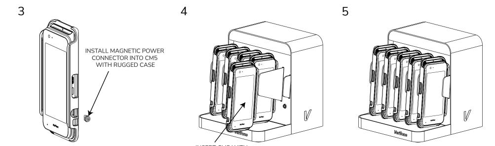
INSERT CM5 WITH RUGGED CASE AS SHOWN
